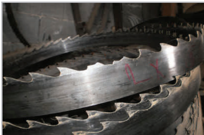
Slika 6. Oštećena pila Figure 6. Damaged saw
